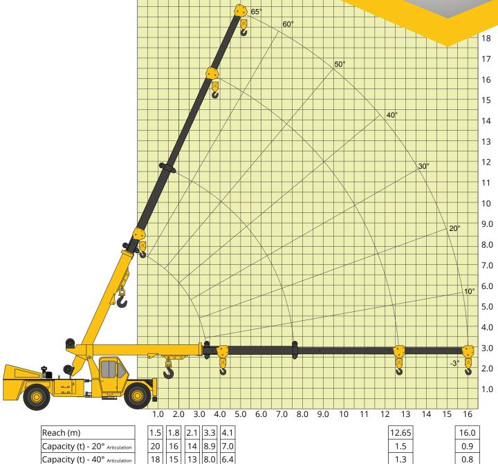
Radius is the horizontal Distance Measured from the center of front wheel to the load point
